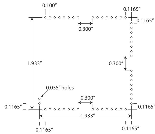
\* hole diameter for SIP size pins is .035"
