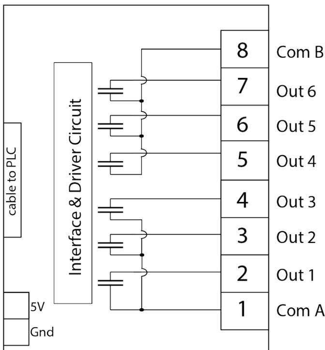
Power must be connected to the two position terminal block labeled GND and +5V. Connect ground to the terminal closest to the module corner and +5VDC to the other terminal, labeled +5V. The ground must be connected to the PLC's ground. When power is properly connected and on, the LED indicator will light.
