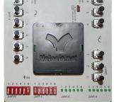
For use with your custom motherboard, the process is basically the same, except that it starts a couple of steps earlier. The eBranch comes with sockets for your motherboard. The sockets are standard 0.1" sockets, designed for use with 0.1" spacing, .025" square post headers. The correct number of 8 pin sockets (for IO) and one two pin socket (for PLC power) come included with the eBranch. An 8 pin version of those sockets is pictured on the right.
