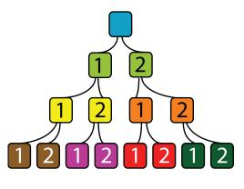
level PLC above it that has a program. If the application places a program in a Branch Expansion, Branch Expansion units that are below it in the tree and configured as IO serve as its expansion IO.
