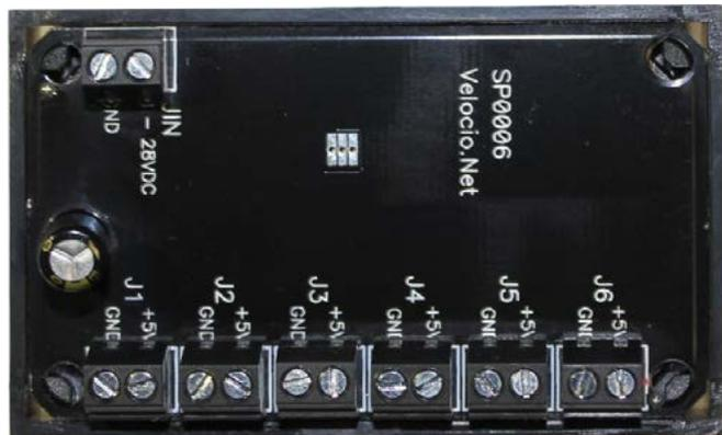
source supply). All output terminals are directly connected, so that current can be distributed in any desired ratio.
